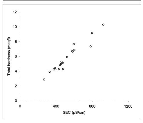
Fig. 2: Relation between total hardness of water and specific electric conductivity.
